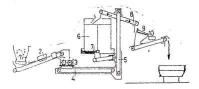
PIcture 11-7: The technological scheme of the process: 1-storage hopper; 2-magnetic strip separator; 3-hammer crushing installation; 4-(vibrating) belt conveyor; 5-elevator; 6-4 chamber maturizer (hygienizer); 7-screw dispenser; 8-belt conveyor; 9screen; 10- magnetic separator.
