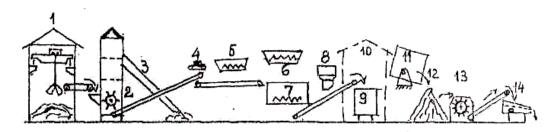
*Picture 11-2:* **Prat-Sofraine procedure**. 1-bunker; 2- hammer crusher; 3- infrared separator; 4magnetic separator; 5- compost dispenser; 6- domestic sludge dispenser; 7- mixer; 8- chemical reagents basin; 9- maturation cells; 10- cell storage bay; 11- cell discharge system by tilting; 12posterior maturation prism; 13- grinding installation; 14- screen rotating drum.
