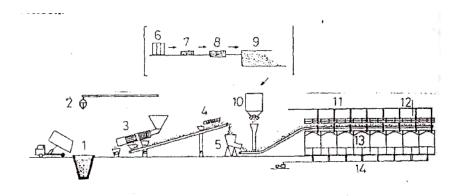
Picture 11-4: The technological scheme of the Humusol-Cifal procedure: 1-bunker; 2- grapple crane; 3- rotating drum screen; 4- magnetic separator; 5-hammer crusher; 6waste waster sludge dispenser; 7-mixer; 8-mixer; 9-seeding material storage cell; 10-dispenser; 11, 14-water installation; 12-movement area; 13-maturation cells.
