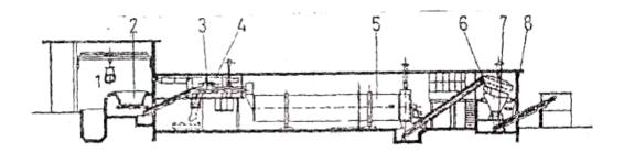
Figura 11-6: The technological scheme of Dano biostabilization procedure: 1-storage hopper and grapple crane; 2-dispenser; 3- magnetic separator; 4-manual sorting strip; 5- maturation drum (biostabilizer); 6-vibrating screen; 3- hammer crushing installation; 8- belt conveyor for discharging the screen scraps.
