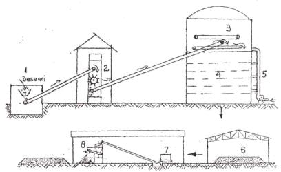
Picture 11-5: Thompson (Carel-Fouché) procedure technological scheme: 1-storage hopper; 2-hammer crushing installation (Gondard); 3-distribution strip; 4maturation tower; 5-venting installation; 6-subsequent maturation; 3-dosing tank; 8subsequent screening.
