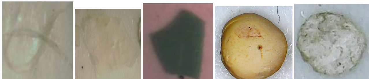
Figure 17 - Examples of the shapes of microplastics found in the Sulina and Casla Vadanei beach; From left to right: filament, film, fragment, pellet, foam. (Original Photos: INCDM, Constanta, Romania)
