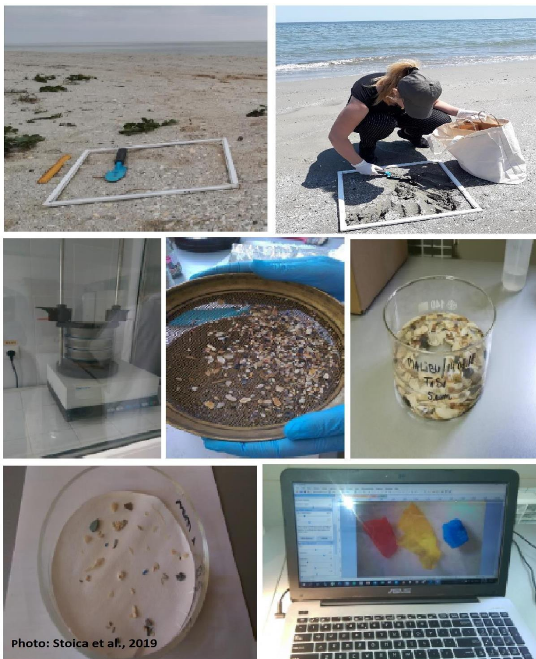
Figure 8 Figure 9. Flow diagram for the analysis of microplastics in beach samples (Sulina and Casla Vadanei) Results and discussion
